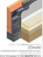
90mm Kingspan K106 λ0.019 90mm Celotex Thermaclass 21 λ0.021 90mm Unilin Cavity Fill XT/CF λ0.021
